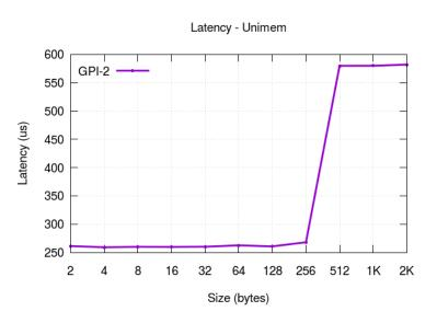
Performance results of two Trenz-Prototype-Boards@Forth connected via UNIMEM
